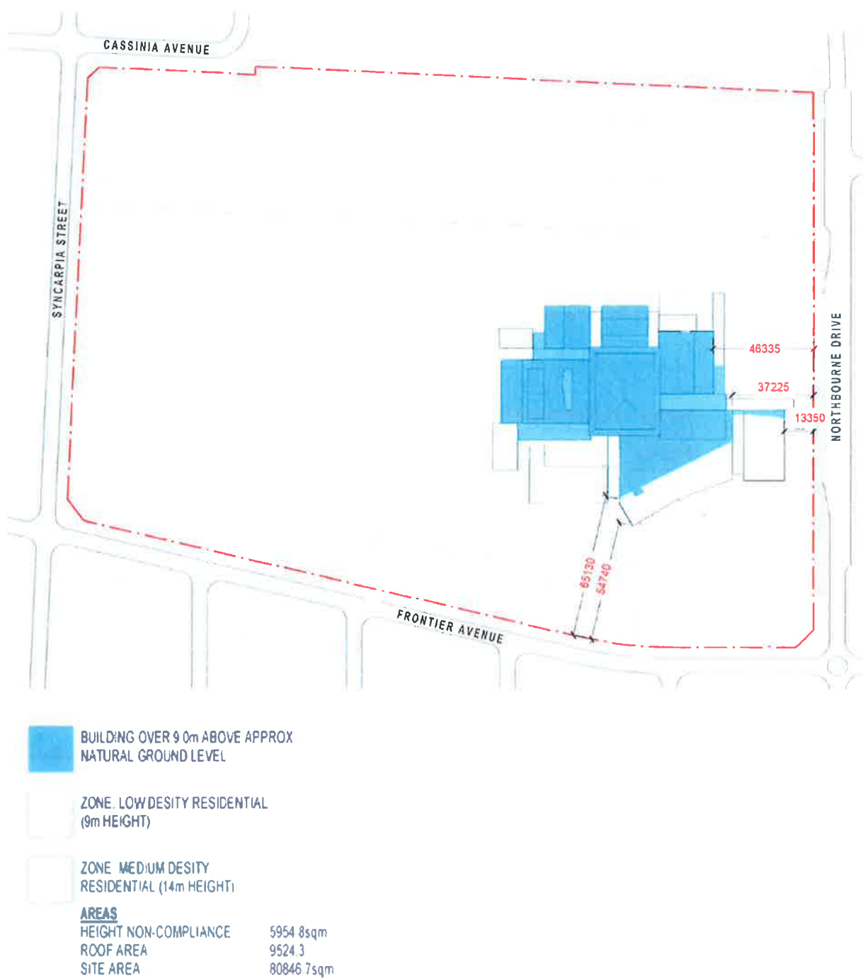
Figure 2 – Proposed non-compliance with the 9m height of buildings standard (in plan)
